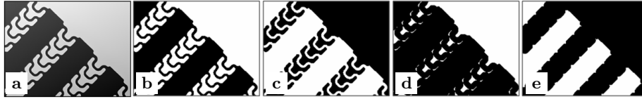
Fig. 2. The results of the intermediate steps of calculating the mean channel depth. Left to right: (a) Raw image – (b) Segmentation of upper surface – (c) Segmentation of channel layer – (d) Erosion of (b) – (e) Erosion of (c).
