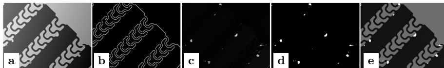
Fig. 5. Results of the main processing steps for defect detection. Left to right: (a) Raw image – (b) Morphological gradient – (c) Difference of model and acquired image – (d) Opening of (c) – (e) Chip image with detected defects overlaid in white (originally, defects are shown in color).
