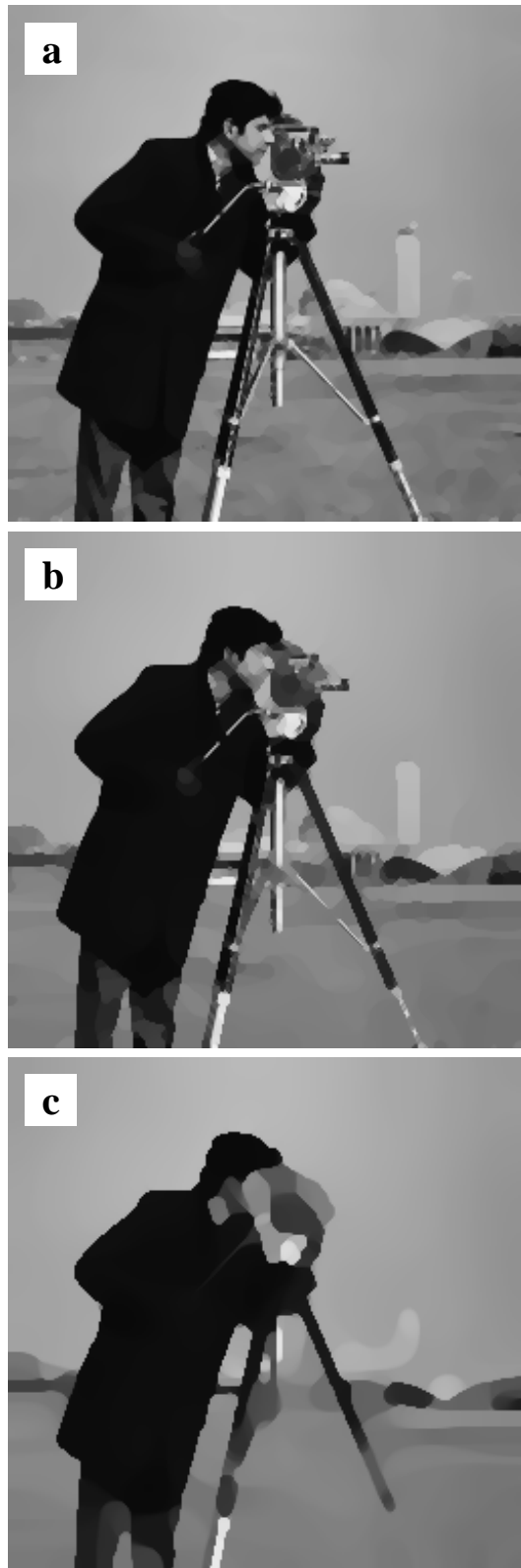
Fig. 5 The Cameraman experiment with self-snakes. An edge-stopping function of Perona-Malik type (corresponding to the Euclidean amoeba metric) is used. (a) Self-snakes filtering of Fig. 3(a), \sigma = 0.25 , time step 0.25, 67 iterations. (b) Same as in (a) but 267 iterations. (c) Same as in (b) but \sigma = 0.05 .
