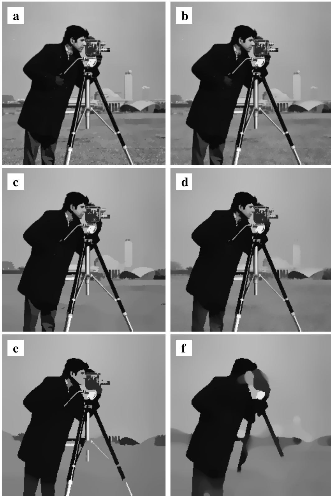
Fig. 4 Iterated amoeba median filtering of cameraman image with different parameters. The Euclidean amoeba distance was used throughout this figure. Top row: (a) \rho = 5 , \sigma = 0.25 , 4 iterations. (b) \rho = 10 , \sigma = 0.25 , 1 iteration. Middle row: (c) \rho = 10 , \sigma = 0.25 , 4 iterations. (d) \rho = 20 , \sigma = 0.25 , 1 iteration. Bottom row: (e) \rho = 20 , \sigma = 0.25 , 4 iterations. (f) \rho = 10 , \sigma = 0.05 , 4 iterations.
