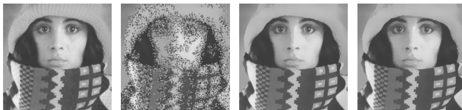
Fig. 2. Influence of the numerical scheme on the result of FAB diffusion ( \lambda = 4 , \kappa = 2.5 , t = 10 ). From left to right: (a) Test image, 256 \times 256 pixels. (b) Explicit scheme (3) with standard discretisation (5). Computing 1 million iterations with time step size \tau = 10^{-5} requires 70 minutes and 13 seconds, while the result is unstable. (c) Explicit scheme (3) with nonstandard discretisation (5). Performing 1 million iterations with \tau = 10^{-5} takes 66 minutes and 34 seconds. (d) Corresponding two-pixel scheme. We used 100 iterations with synchronisation step size \tau_{\max} = 0.1 , leading to a runtime of 7.73 seconds. The average time step size was 0.0991.
